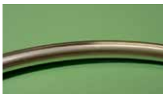
Figure 2: Parker Hannifin's Silver-Indium diffused plating
